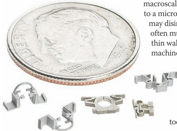
Thin-wall microparts prove difficult to EDM because the walls sometimes disintegrate. Shown are fiber-optic clips with 0.100mm-thick walls. The parts at left required two operations and were rotated 90° in a fixture accurate to within 2µm.
