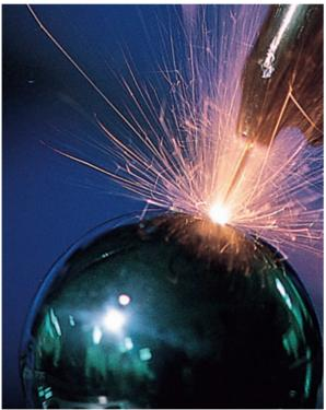
Small-hole EDMing is performed with a spinning electrode. Shown is a 0.040"-dia. hole being EDMed in a 0.5000"-dia. ball bearing.
